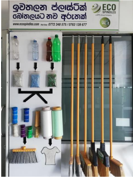
Image 2: End products produced from the recycled plastics by Eco spindles. (Eco Spindles (PVT) Ltd., 2020)
